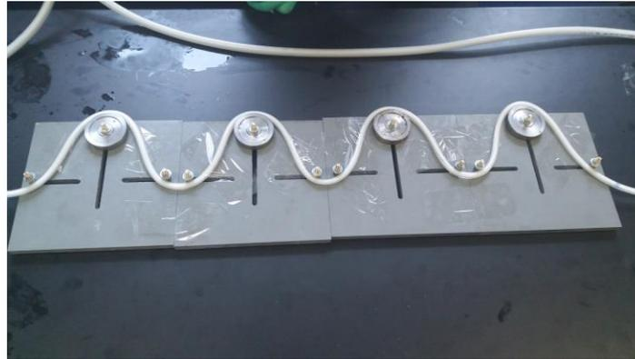
**Figure 1:** A coronary tortuosity model with tube and simulate blood pumping by heart pumping machine
