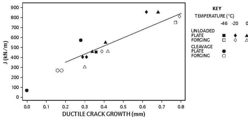
**Figure 3** : Fracture Toughness,  $J$ , of Plate and Forging as a Function of Ductile Crack Growth
