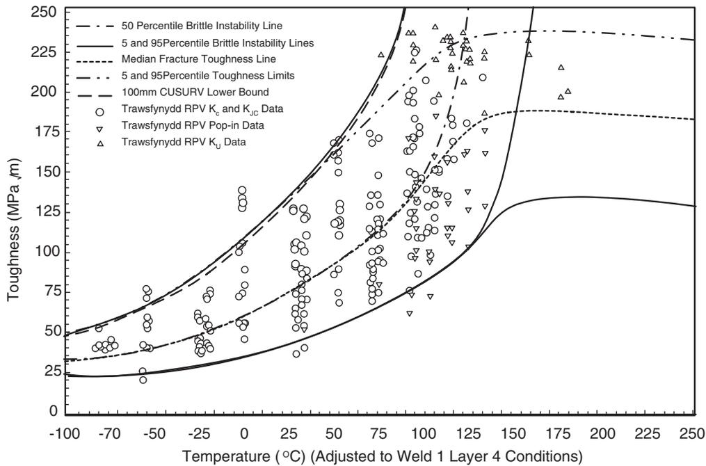
**Figure 4** : Fracture toughness data,  $K_c$  or  $K_{Jc}$  obtained for C-Mn submerged arc weld metal obtained from a decommissioned Trawsfynydd pressure vessel as function of temperature compared with the CUSURV prediction.
