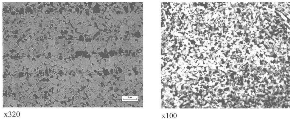
**Figure 1** : Optical Micrographs of C-Mn Steel a) Forging and b) Plate showing Ferrite and Pearlite (etched in Nital)
