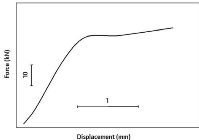
**Figure 2** : Example of a Force Displacement Curve Obtained on a Forging Specimen at  $-46^{\circ}\text{C}$ .
