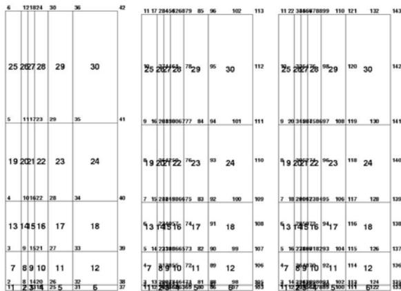
(a) 4-noded (b) 8-noded (c) 9-noded
