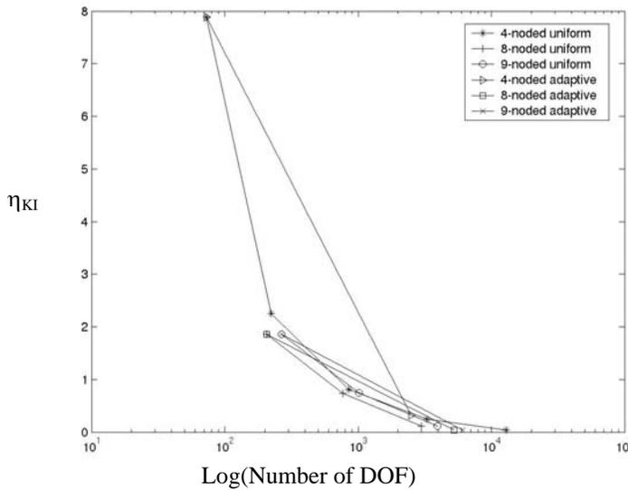
**Figure 8 :** Convergence of Uniform and Adaptive Meshes (Mode I - Centre Crack)
