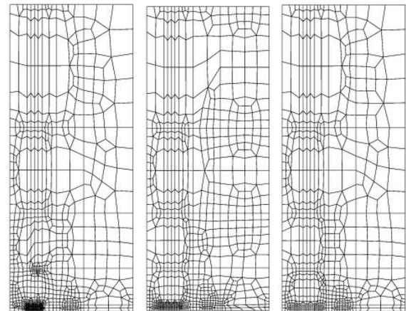
(a) 4-noded (b) 8-noded (c) 9-noded
