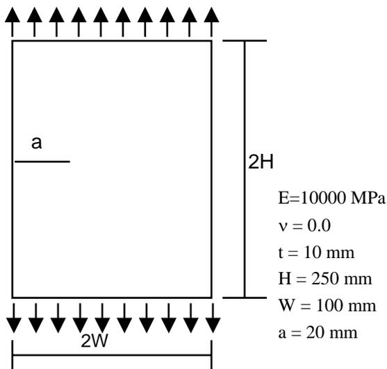
**Figure 9 :** Rectangular Plate with Edge Crack
