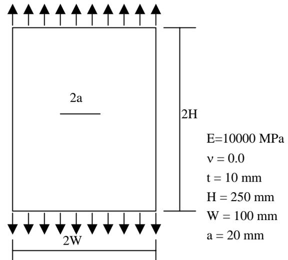
Figure 3 : Rectangular Plate with Center Crack
