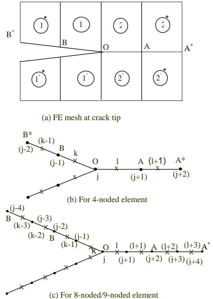
**Figure 2 :** Details of FE Mesh at Crack Tip Region for Improved SERR Evaluation
