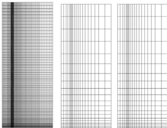
(a) 4-noded (b) 8-noded (c) 9-noded
