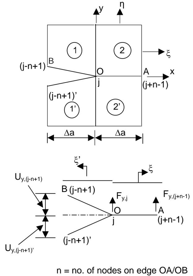
Figure 1 : Typical FE Mesh of Crack Tip Region
