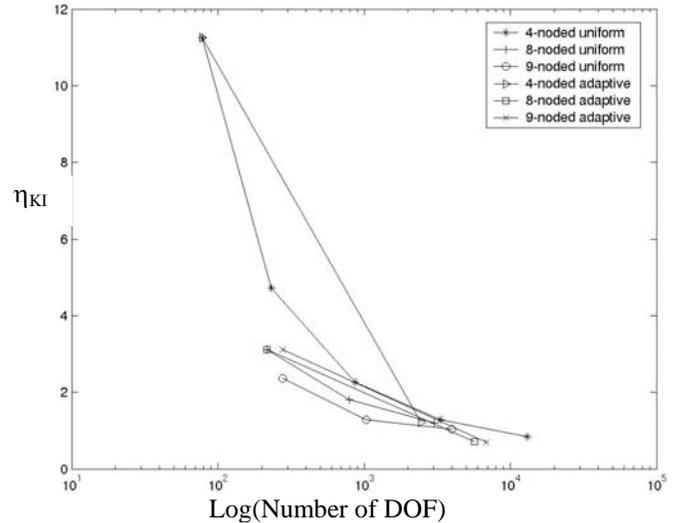
**Figure 11 :** Convergence of Uniform and Adaptive Meshes (Mode I - Edge Crack)
