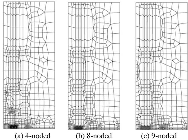
**Figure 10 :** Adaptive Mesh Employed in the Studies (Mode I - Edge Crack)
