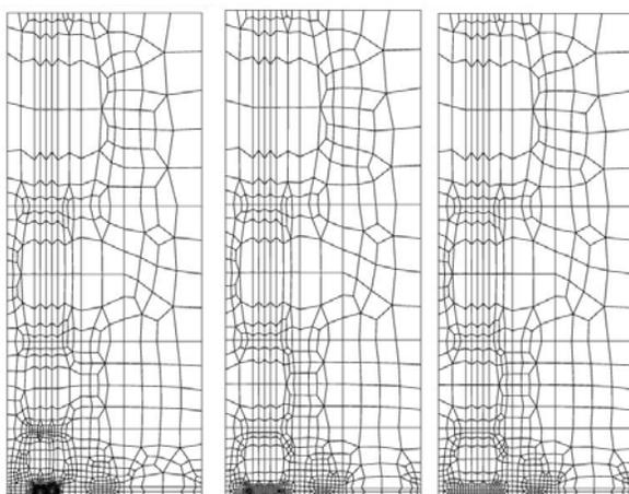
(a) 4-noded (b) 8-noded (c) 9-noded
