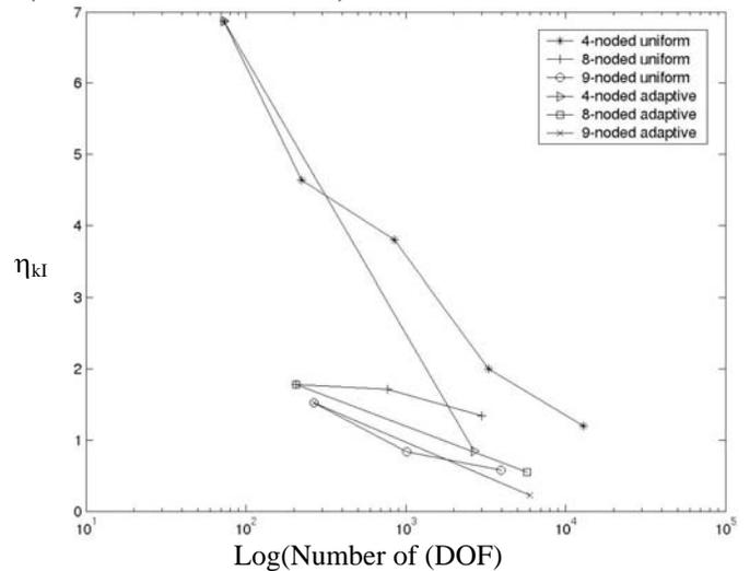
Figure 14 : Convergence of Uniform and Adaptive Meshes (Mode II - Centre Crack)
