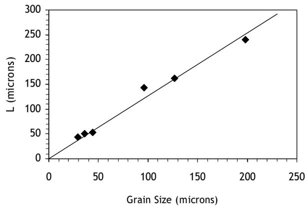
**Figure 9** : L values calculated from the data of Yokobori and Konusu (1977), plotted as a function of the grain size of the material.
