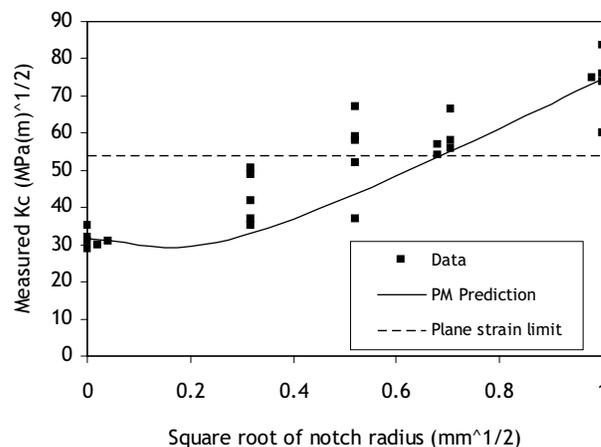
**Figure 5** : Data from Tsuji et al (1999) on low-temperature cleavage fracture of steel. Predictions using the PM (with  $L=0.05\text{mm}$ ); plane strain limit value calculated using equation 7.
