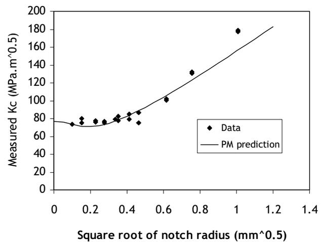
**Figure 8** : Data [Mulherin, Armiento and Marcus (1963)] and PM predictions for an aluminium alloy tested under plane stress conditions.
