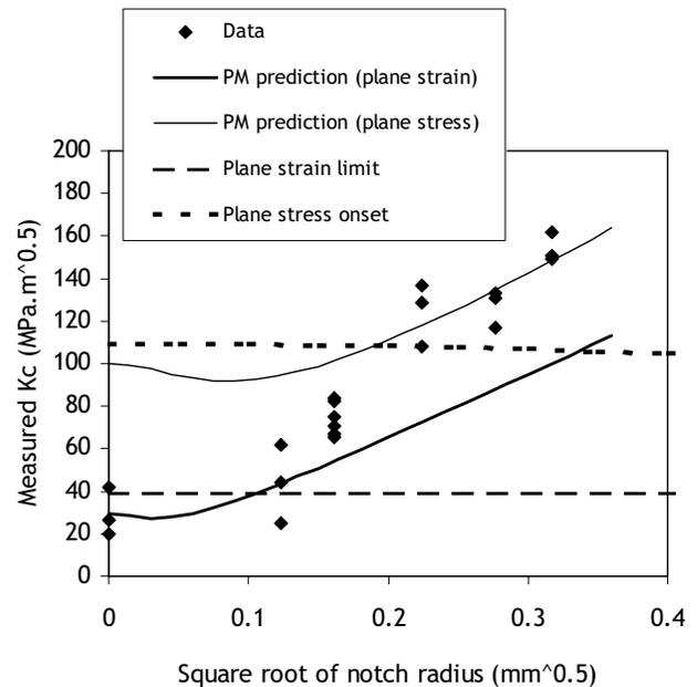
**Figure 7** : Data on a high-strength steel tested at room temperature [Irwin (1964)], showing the plane strain limit, plane stress onset and some possible PM predictions for plane strain and plane stress.
