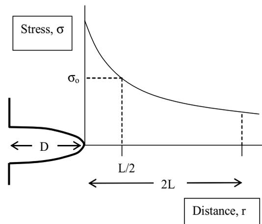
**Figure 1 :** A typical notch, with depth  $D$  and root radius  $\rho$ . TCD methods use the stress/distance curve: for the Point Method (PM), failure occurs when the stress at a distance  $L/2$  is equal to the characteristic strength  $\sigma_0$ ; for the Line Method (LM), failure occurs when the average stress over a distance  $2L$  is equal to  $\sigma_0$ .
