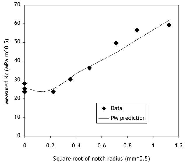
**Figure 3 :** The same data as fig.2, with PM predictions using the optimum value of L ( $0.035mm$ ). Results from FEA were used for the higher notch radii where they differed significantly from those of equation 4. The largest difference between data and predictions is 10.1%.
