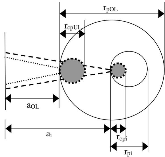
Figure 6 : Wheeler model for tensile-compressive overloads
