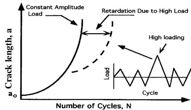
**Figure 1 :** Decrease in the rate of crack growth due to the overload followed by the CAL
