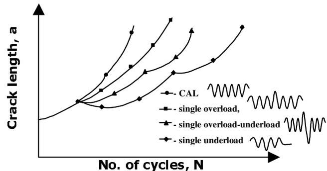
**Figure 2 :** Crack growth produced by (a) CAL, (b) single overload, (c) single overload-underload and (d) single underload
