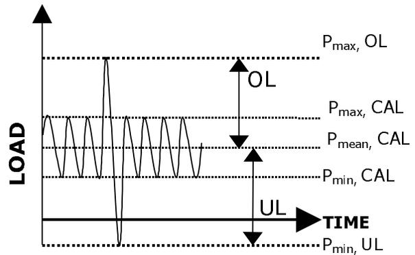
Figure 5 : Schematic diagram of overload and underload
