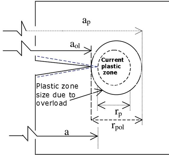
Figure 4 : Wheeler residual stress model
