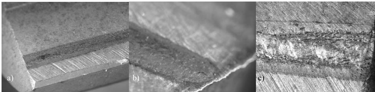
Figure 6 : Pictures of the contact point of the tooth roller-side after tests on casehardened gears
