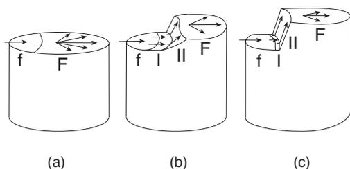
**Figure 9** : Fracture surfaces produced by LAD in steels with different degree of cold drawing: (a) null or slight drawing; (b) intermediate drawing; (c) heavy drawing; f: fatigue crack growth, I: mode I propagation; II: mixed mode propagation; F: final fracture.
