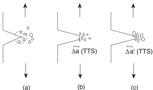
**Figure 6** : Micromechanical model of HAC in hot rolled and slightly drawn steels: the mechanism is the so called *tearing topography surface* or TTS (Thompson and Chesnutt, 1979; Costa and Thompson, 1982) with very closely spaced nucleation of voids or defects.
