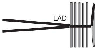
**Figure 12 :** Micromechanical model of LAD in heavily drawn steels, showing chemical crack advance by dissolution and mechanical crack deflection when the macrocrack reaches a pearlitic pseudocolony. The microstructure is assumed to be totally oriented in the cold drawing direction.
