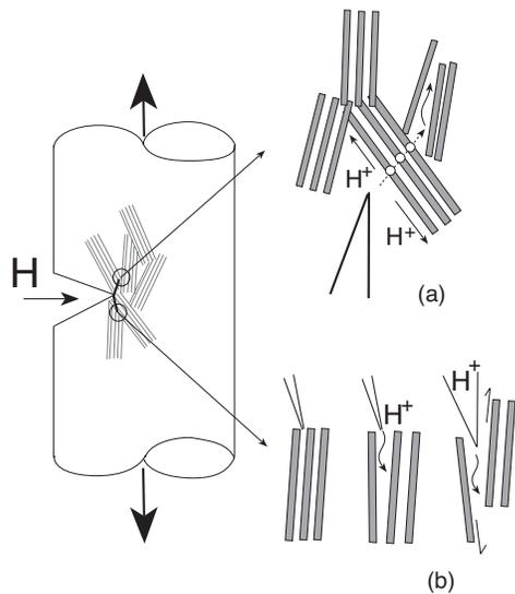
**Figure 7** : Micromechanical model of HAC in steels with an intermediate degree of drawing: (a) hydrogen diffusion in the pearlitic microstructure and penetration along the path opened by a Miller-Smith mechanism of shear cracking (SC); (b) fracture by hydrogen enhanced delamination or debonding (HEDE).
