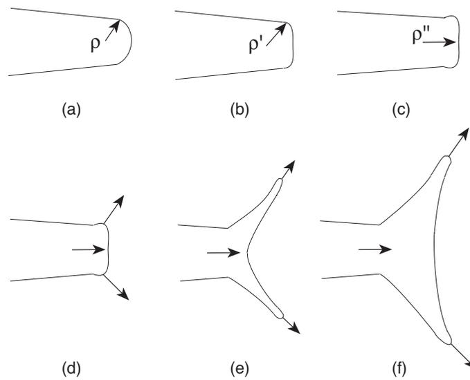
**Figure 11 :** Micromechanical model of LAD which produces crack tip blunting in steels with an intermediate degree of drawing. The figure shows the evolution from smooth blunting (a) to cornered blunting (c) which favours crack tip branching, cf. (d) to (f).
