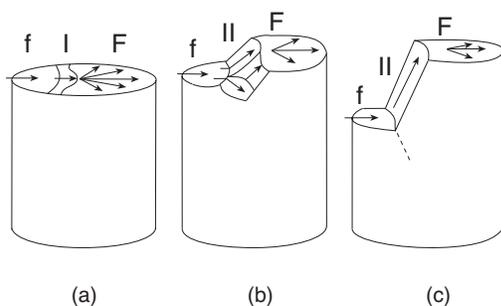
**Figure 5** : Fracture surfaces produced by HAC in steels with different degree of cold drawing: (a) null or slight drawing; (b) intermediate drawing; (c) heavy drawing; f: fatigue crack growth; I: mode I propagation; II: mixed mode propagation; F: final fracture.
