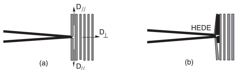
**Figure 8** : Micromechanical model of HAC in heavily drawn steels: (a) hydrogen diffusion in longitudinal and transverse directions; (b) fracture by hydrogen enhanced delamination or debonding (HEDE). The microstructure is assumed to be totally oriented in the cold drawing direction.
