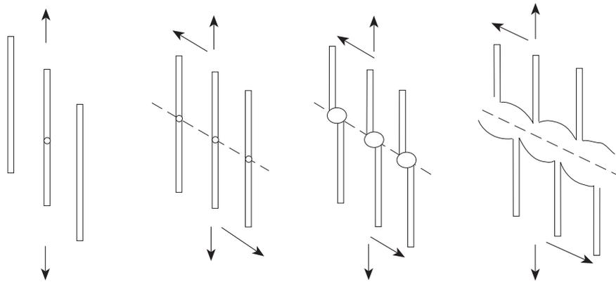
**Figure 3** : Micromechanical model of fracture by shear cracking in pearlitic microstructures (after Miller and Smith (1970)) applicable to fracture in hot rolled and slightly drawn steels. The cementite lamellae are fractured by shear deformation of the ferrite plates. Externally applied stress (vertical direction) and microstructure-induced shear strain are drawn.
