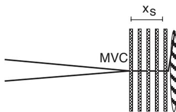
**Figure 4** : Micromechanical model of initiation and final fracture in heavily drawn steels. The microstructure is assumed to be totally oriented in the cold drawing direction;  $x_s$ : mode I propagation produced by micro-void coalescence (MVC).
