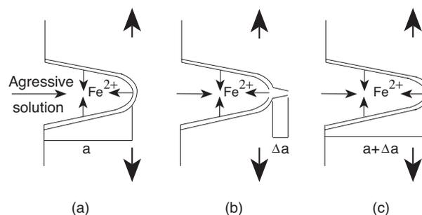
**Figure 10** : Micromechanical model of LAD in hot rolled and slightly drawn steels: (a) initial stage, (b) dissolution, film rupture and crack advance, (c) new loop of dissolution.
