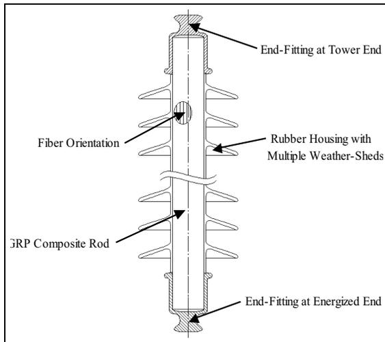
Figure 1: Schematic of a composite suspension insulator
