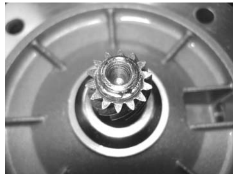
Figure 4: Pinion with a notch in the tooth root
