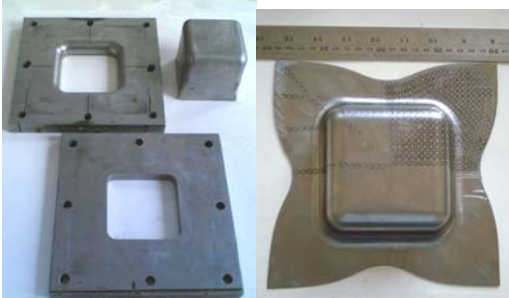
Figure 12: (a) Die set components; (b) Drawn blank
