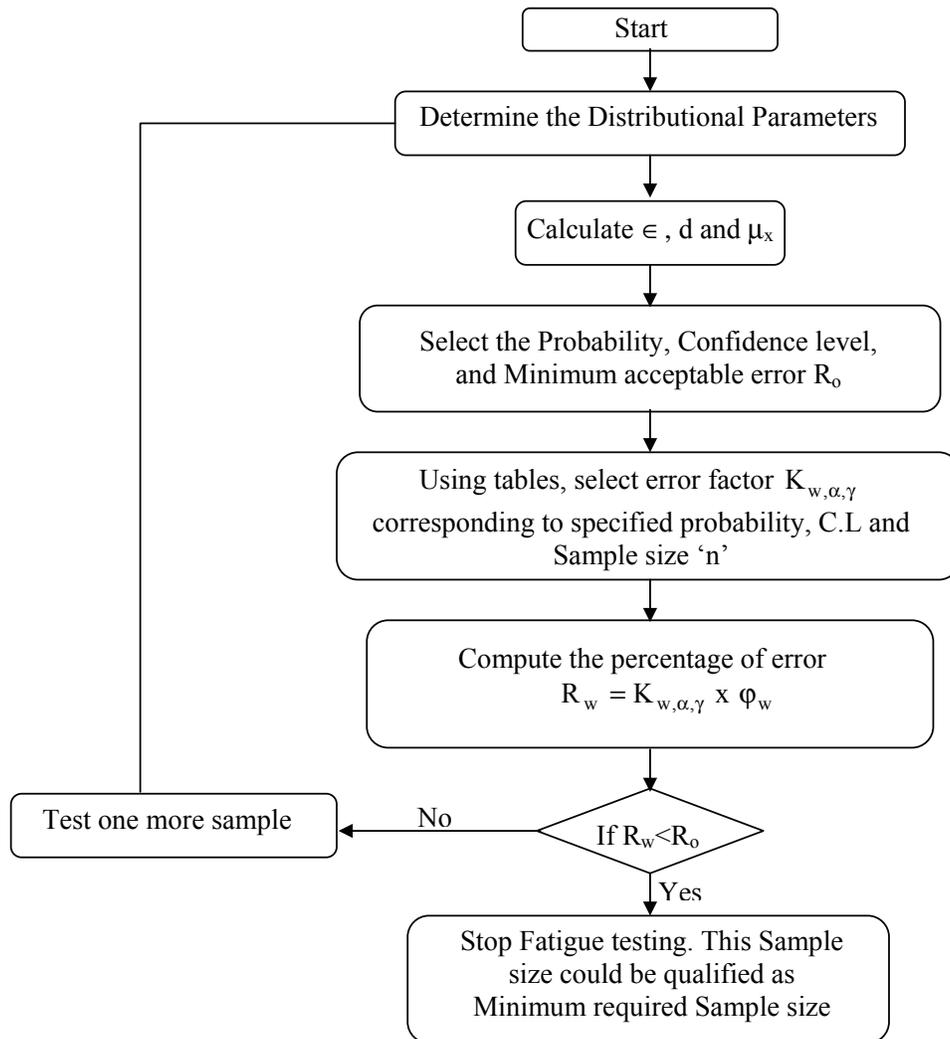
Figure 4: Flow chart for determination of minimum sample size
