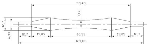
Figure 1: Rotating bending fatigue test specimen (All dimensions are in mm)
