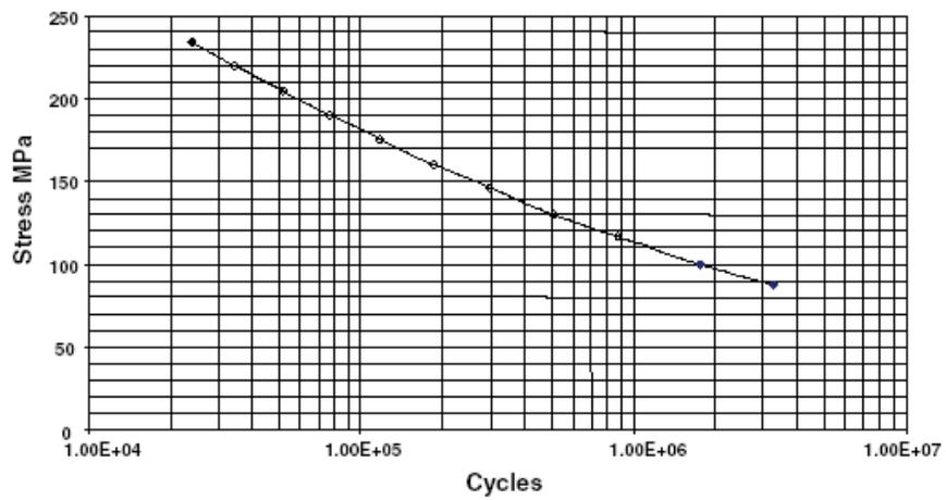
Figure 6: S-N curve of A356.2 material
