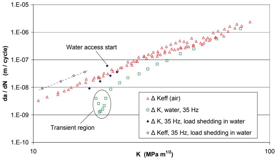
Figure 7: CFCG rates in aqueous environment at load frequency 35 Hz
