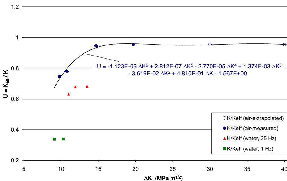
Figure 4: Dependence of U-ratio on actual stress intensity factor range  $\Delta K$
