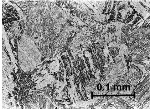
Figure 1: Highly tempered martensitic microstructure of the steel
