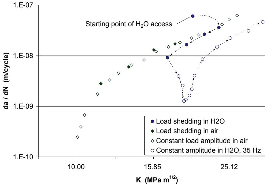
Figure 8: Detail of CFCG behaviour in transient regions in aqueous environment at load frequency 35 Hz
