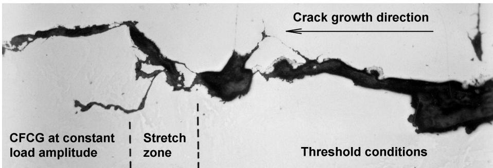
Figure 6: Oxide debris in threshold and FCG regions on specimen longitudinal cut
