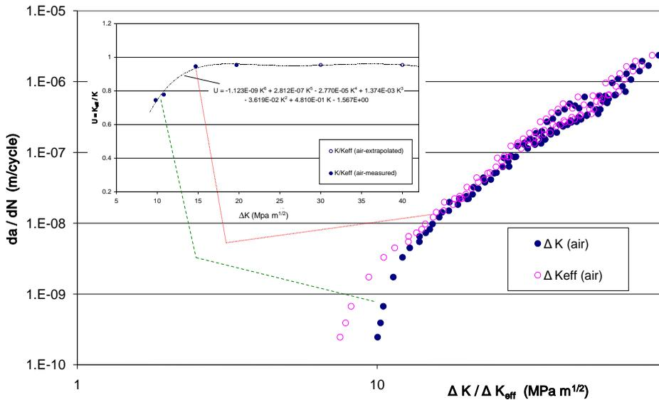
Figure 3: Fatigue crack growth rates in air
