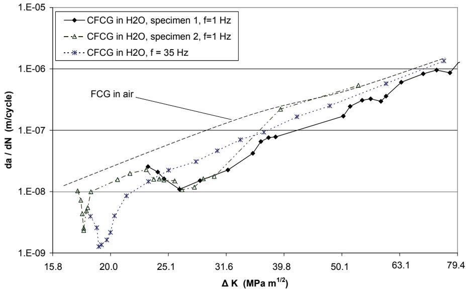
Figure 10: Detail of irregular CFCG in aqueous environment at load frequency 1 Hz
