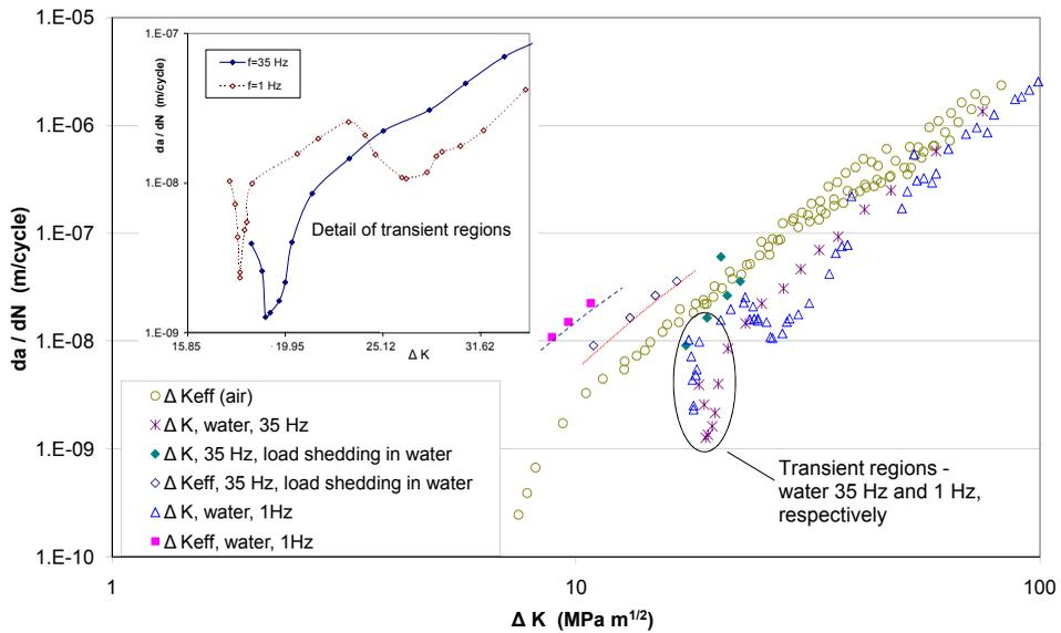
Figure 9: CFCG rates in aqueous environment at load frequency 1 Hz in comparison with other results
