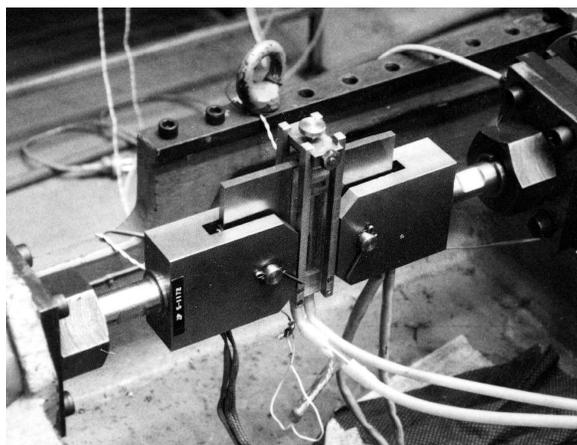
Figure 2: General CT-specimen with attached water chamber
