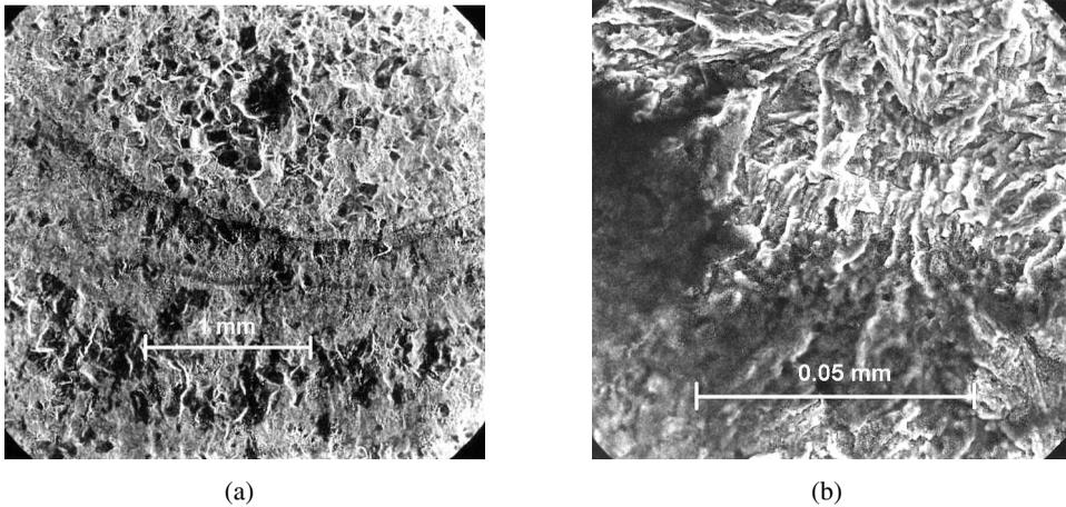
Figure 5: Oxide debris layer of considerable thickness due to fretting corrosion in near threshold region in air, a) total view of crack front, b) detail
