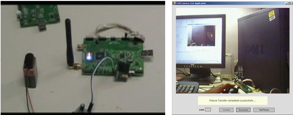
Figure 10: (left) Wireless Image Sensor module in work, (right) Remote desktop server processing captured images.
