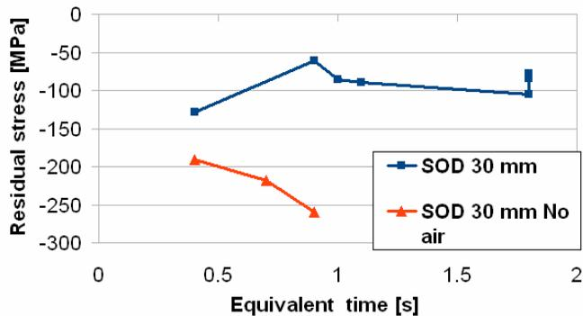
Figure 10: Comparison between submerged WJP with and without air intake ( $SOD = 30$  mm)
