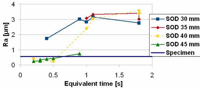
Figure 12: Investigation on roughness improvement in case of submerged WJP with air intake
