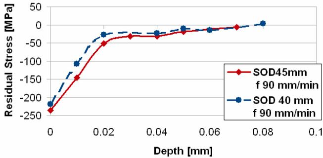
Figure 8: Residual stress distribution along thickness
