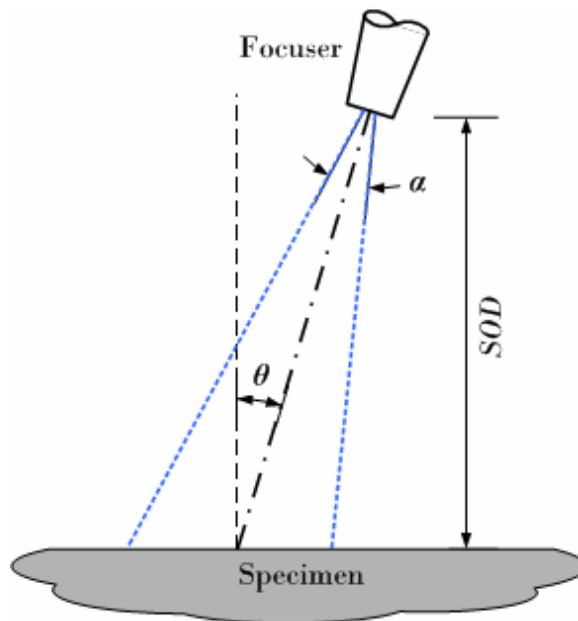
Figure 2: Geometry of the water jet in air Hashish et al (2005)
