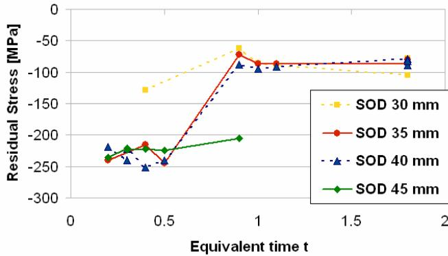
Figure 7: Results for submerged WJP with air intake
