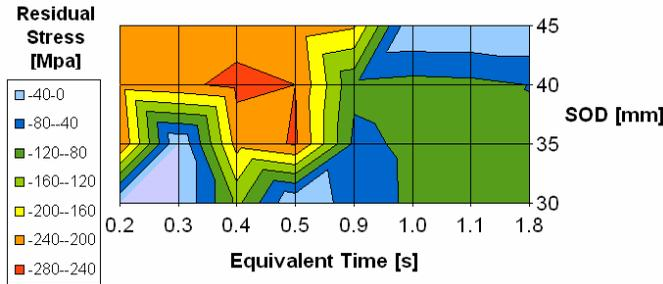
Figure 9: Residual stress map for submerged WJP with air intake
