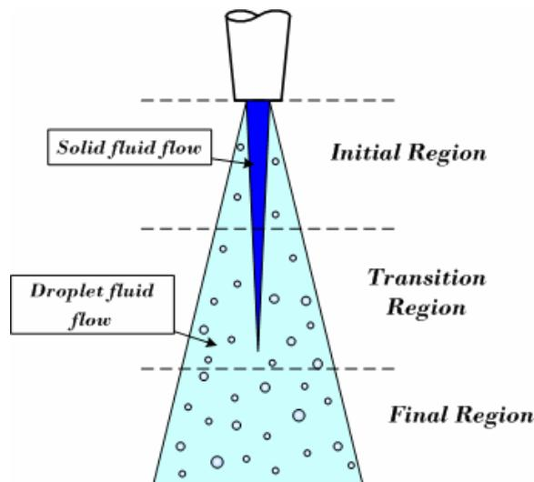
Figure 1: Morphology of a pure water jet in air Yanaida, K.; Ohashi, A. (1978); Yanaida and Ohashi (1980).
