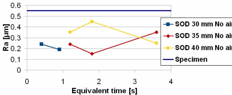
Figure 13: Investigation on roughness improvement in case of submerged WJP without air intake
