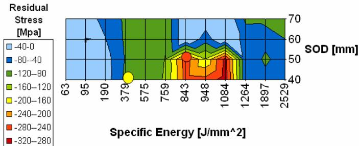
Figure 6: Residual stress map for WJP in air
