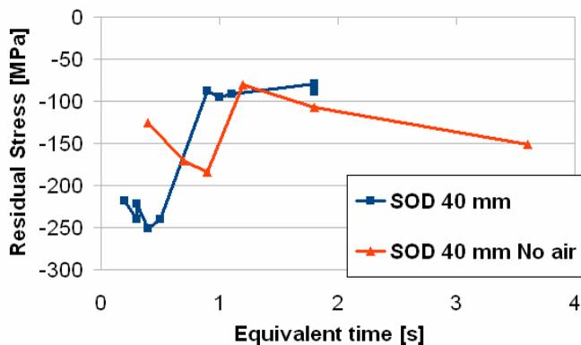
Figure 11: Comparison between submerged WJP with and without air intake ( $SOD = 40$  mm)
