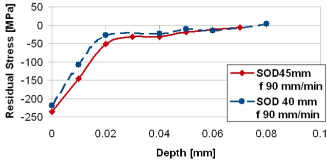
Figure 8: Residual stress distribution along thickness
