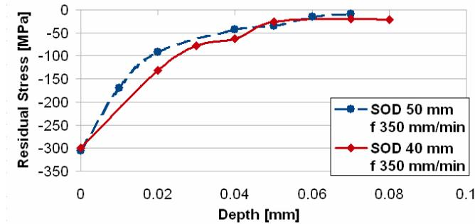
Figure 5: Residual stress distribution along the thickness for WJP in air
