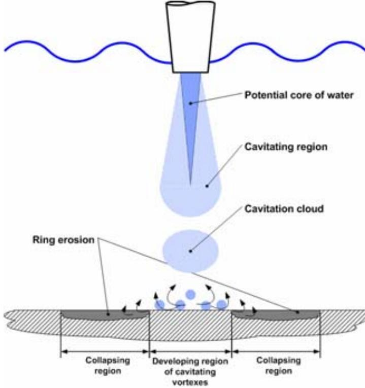
Figure 3: Morphology of the submerged water jet Park et al (2000)
