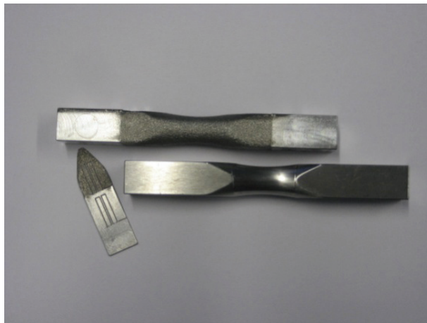
Figure 3: View of the treated, untreated specimens and the slice cut by EDM
