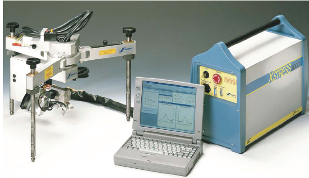
Figure 2: AST X-Stress 3000 X-ray diffractometer used for residual stress measurements
