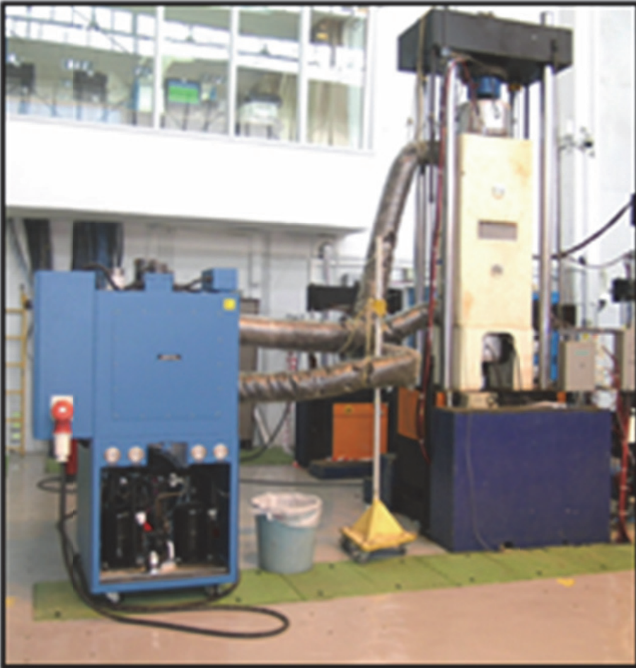
Figure 6: Test set-up for the Carbon-Epoxy Reinforced Panel Tested at -50^{\circ}\text{C}
