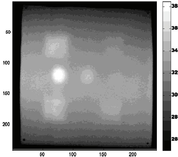
Figure 2: Contour Map of thermogram acquired 20 sec from the start of cooling transitory.
