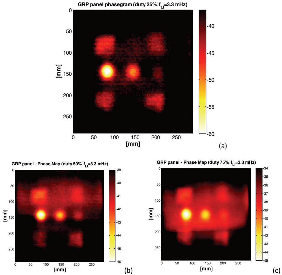
Figure 9: Phase maps from the GRP sample obtained at a Lock-In correlation frequency of 3.3 mHz, and heat deposition modulated with duty cycles of: a) 25%; b) 50%; c) 75%.
