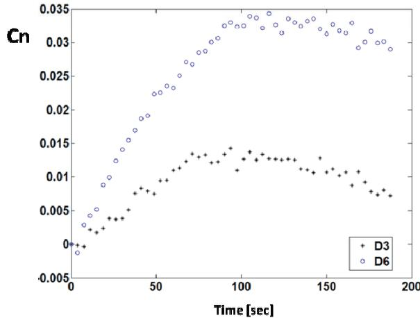
Figure 4: Comparison of Normalised Contrast for defects D3 and D6 (Teflon patch vs blind back hole).
