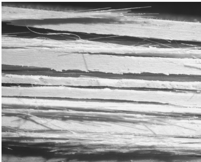
Figure 10: Delamination of a specimen (MAT3)
