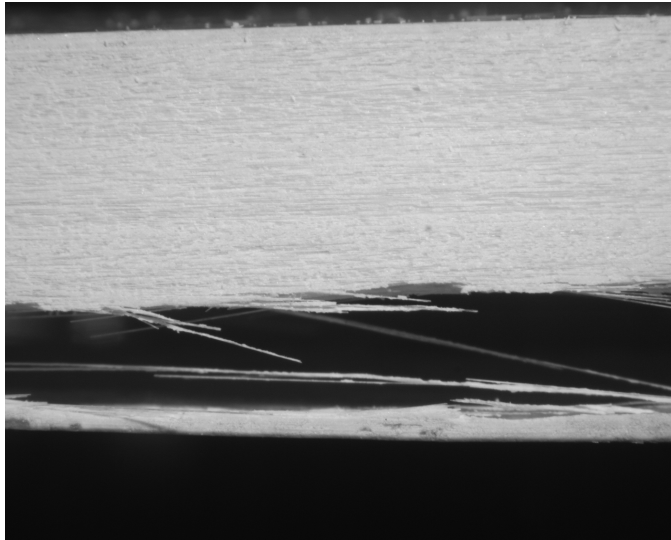
Figure 9: Delamination of a specimen (MAT2)
