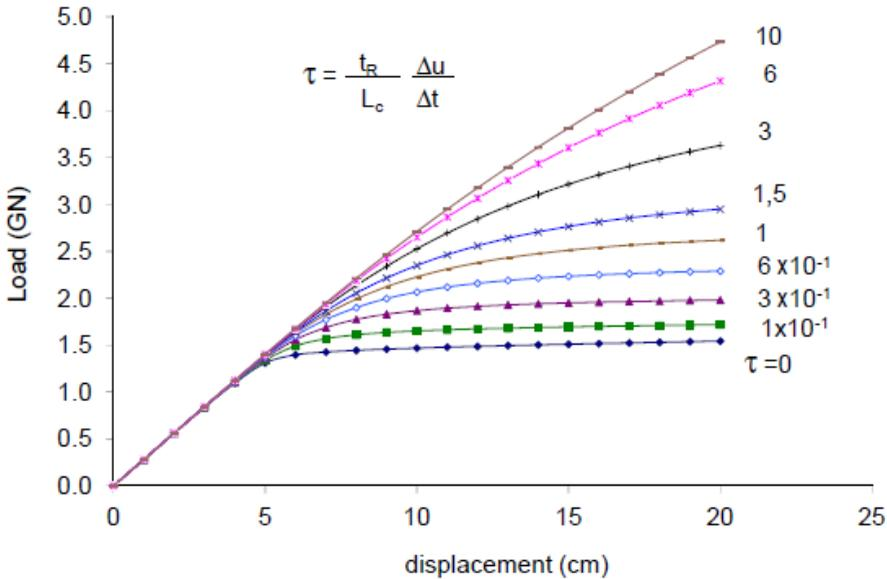
Figure 3: Perforated strip: load vs. displacement curves.
