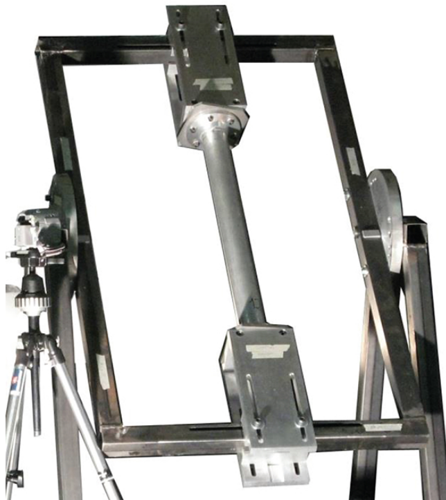
Figure 1: Experimental set up of the ballistic test: the shaft specimen is 45^\circ oriented respect to bullet trajectory
