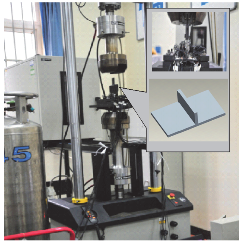
Figure 8: Tensile testing machine and T-joint reinforced plate specimen.
