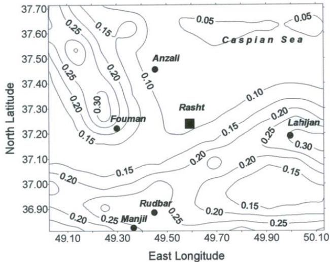
Figure 2: Horizontal seismic hazard (PGA over bedrock) map of Guilan province using logic tree for a 475-year return period [Amiri and Amrei (2008)].
