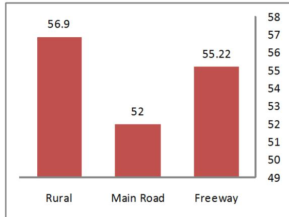
Figure 6a: Average SHM score of abutment in single span bridges (out of 60).
