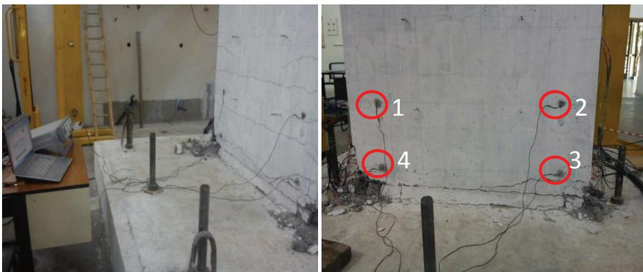
Figure 3: (b) Experimental setup and (c) Location of for PZT patches.
