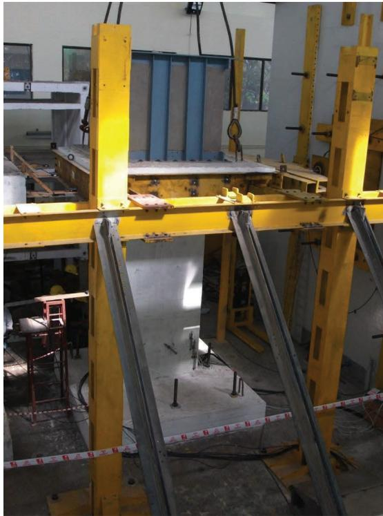
Figure 3(a): Experimental setup for the cyclic load test on shear wall.
