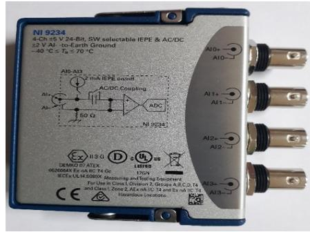
**Figure 2:** Data Acquisition Hardware-NI9234-4 Channel DAQ
