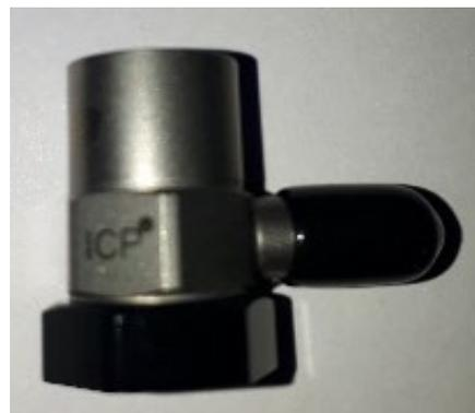
**Figure 3:** IEPE type Accelerometer
