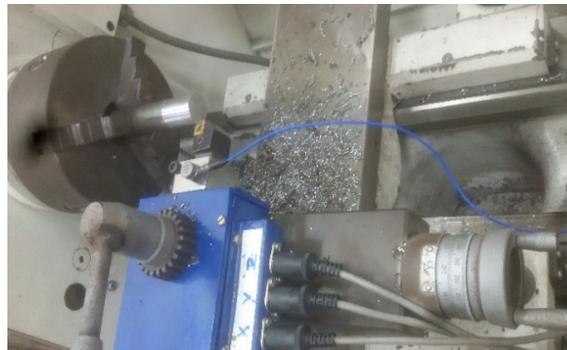
**Figure 1 (b):** Sensor attached to the tool post
