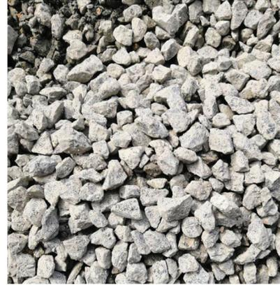
**Figure 3:** Particle size of 10~20 mm
