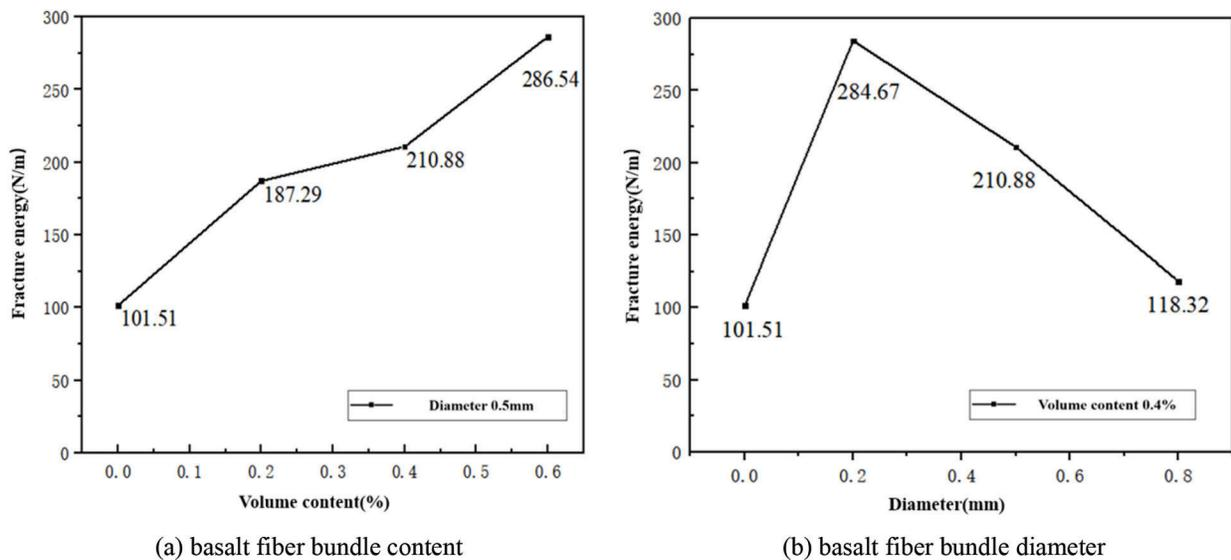
**Figure 9:** The relationship between fracture energy and basalt fiber bundle content and diameter
