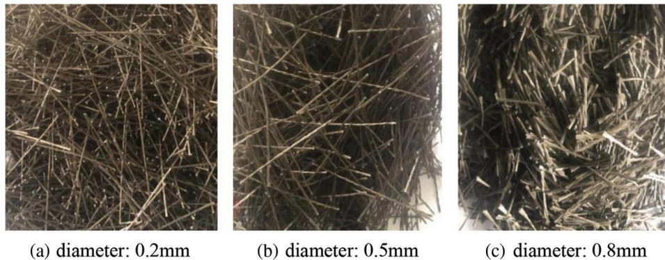
**Figure 1:** Basalt fiber bundles of different diameters Adapted with permission from reference [25], Copyright © 2022, Journal of Physics: Conference Series
