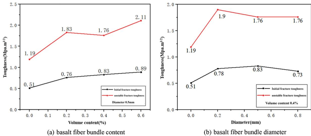
**Figure 6:** The relationship between fracture toughness and basalt fiber bundle content and diameter
