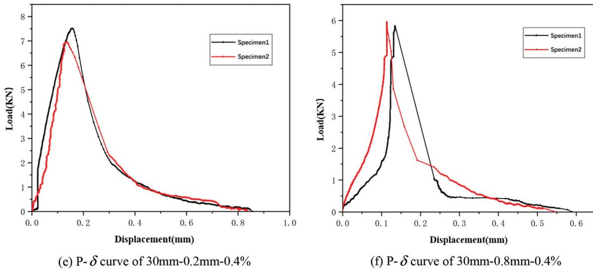
**Figure 8:** The mid-span load-displacement curves of the specimens
