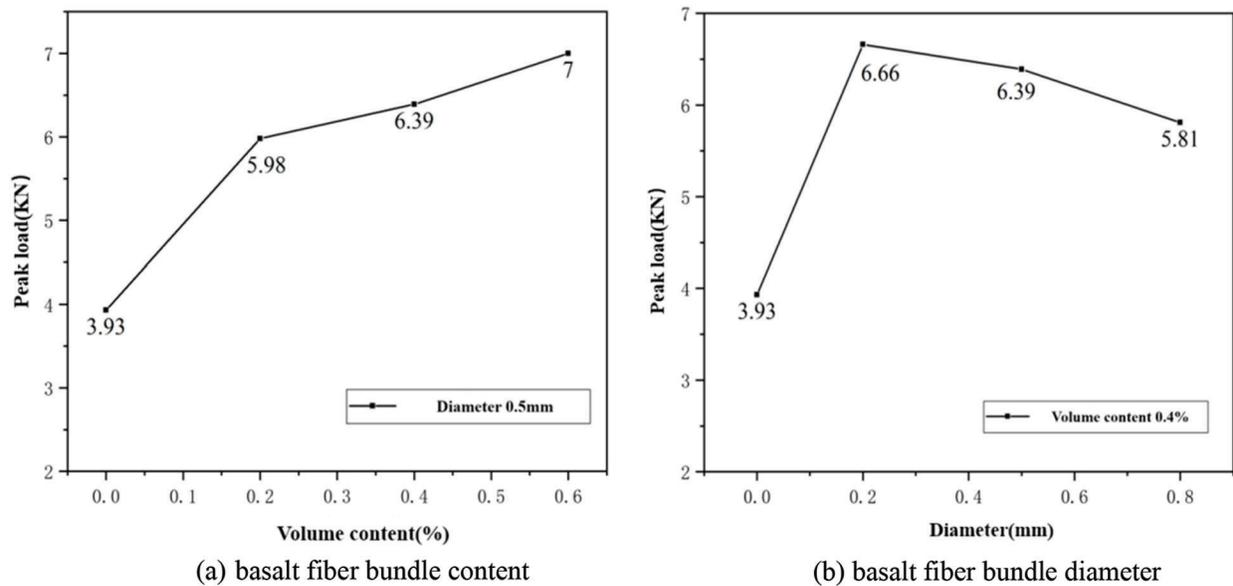
**Figure 7:** The relationship between peak load and basalt fiber bundle content and diameter
