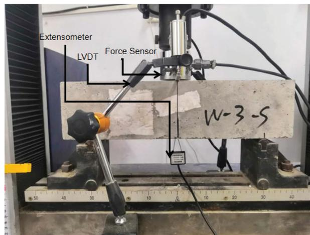
**Figure 4:** Loading device for fracture test
