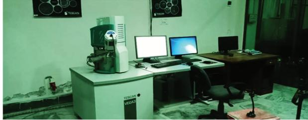
**Figure 1:** SEM for morphological investigation of PZT sample
