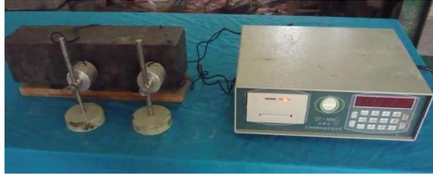
**Figure 2:** Photograph of concrete dynamic elastic modulus measurement
