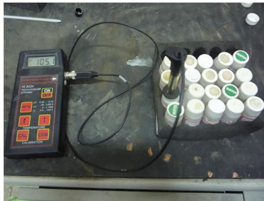
**Figure 3:** Photograph of chloride ion concentration measurement for concrete powder
