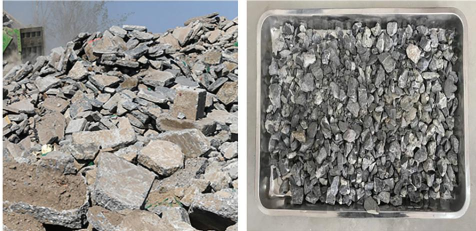
**Figure 1:** Construction waste and recycled coarse aggregate
