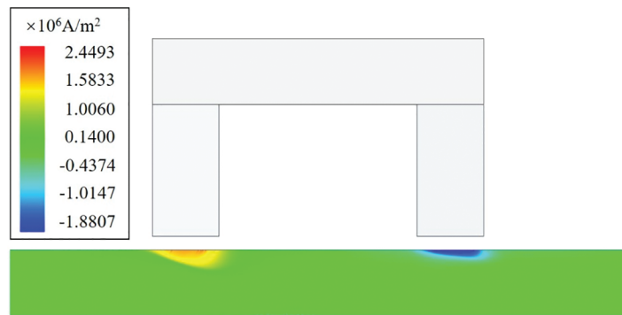
Figure 7: The eddy current distribution at the speed of 1.0 m/s
