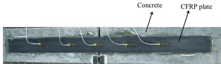
**Figure 13:** Typical example: CFRP externally bonded strengthening for concrete structures
