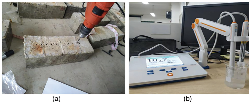
Figure 4: (a) Powder extraction and (b) free \text{Cl}^- ion concentration measurement setups
