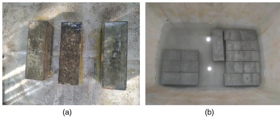
Figure 3: \text{Cl}^- salt erosion of reinforced concrete specimens. (a) Application of epoxy resin adhesive; and (b) immersion of specimens in the 5% NaCl solution
