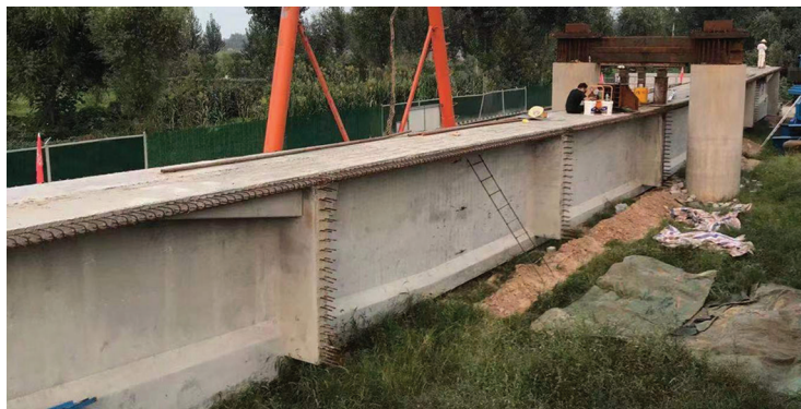
Figure 4: Site diagram of T-beam load loading
