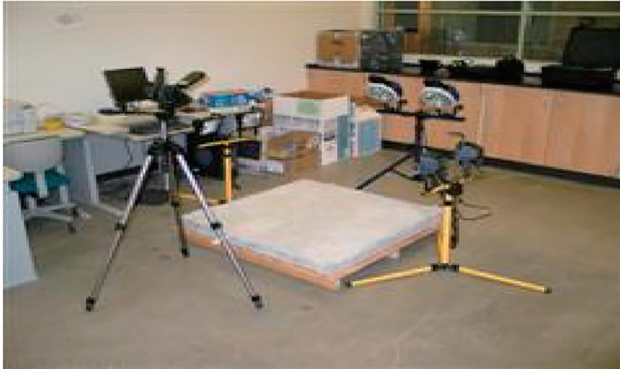
Figure 14: Active IRT experimental setup for defect detection in a concrete slab specimen. Reprinted from Reference [50]
