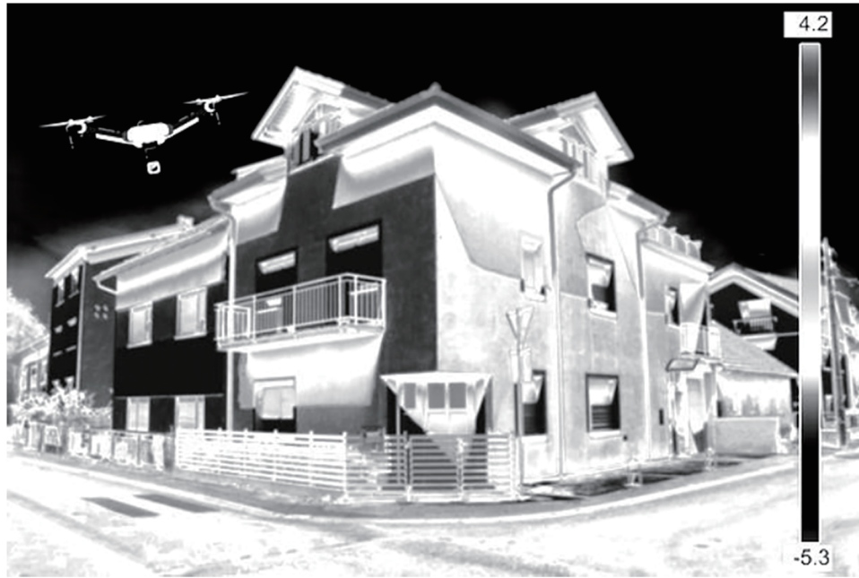
Figure 28: Thermal imaging using a drone. Reprinted from Reference [107]
