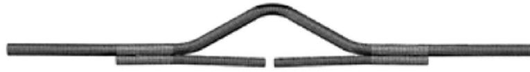
(b) Schematic diagram of weak connection and wave induced steel bar fracture
