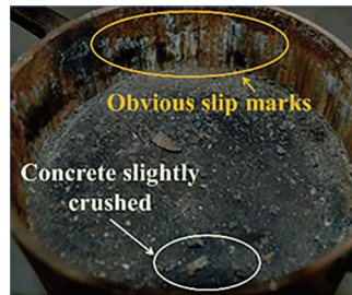
Figure 6: Specimen failure mode diagram
