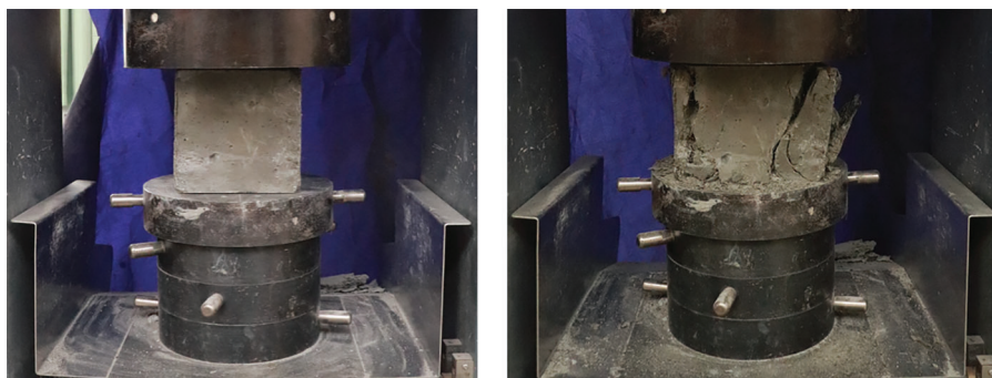
Figure 2: UHPC compressive strength test
