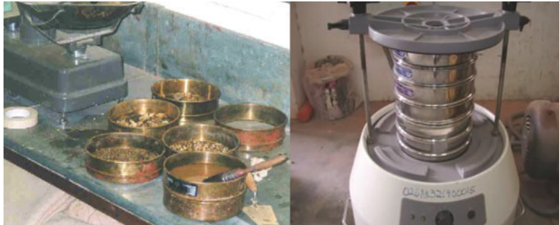
Figure 7: British standard sieve set and mechanical sieve shaker
