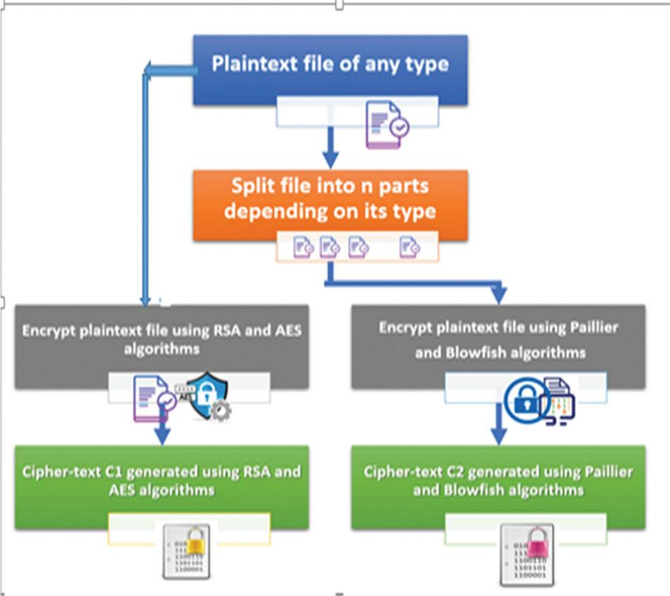
Figure 4: Encryption phase of the hybrid system
