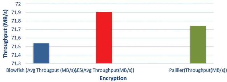
Figure 10: Comparison of average of average throughput for various block ciphering modes
