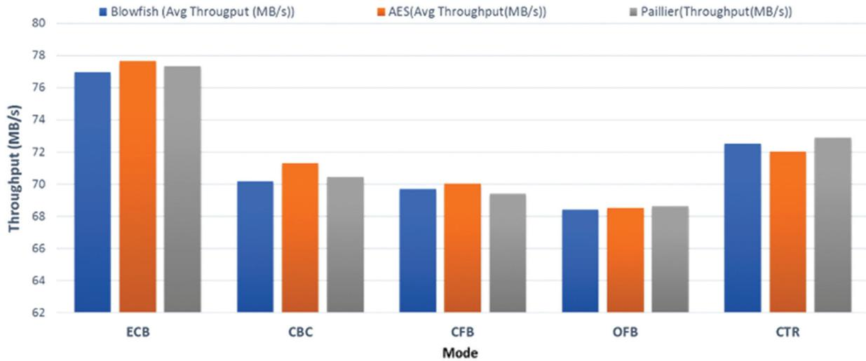
Figure 9: Throughput comparison of various block ciphering modes
