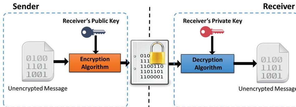
Figure 2: Cryptographic process
