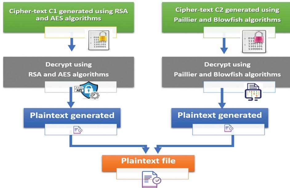
Figure 5: Decryption process of the hybrid system
