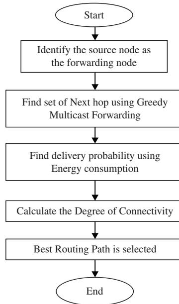
Figure 3: Flowchart for the routing process
