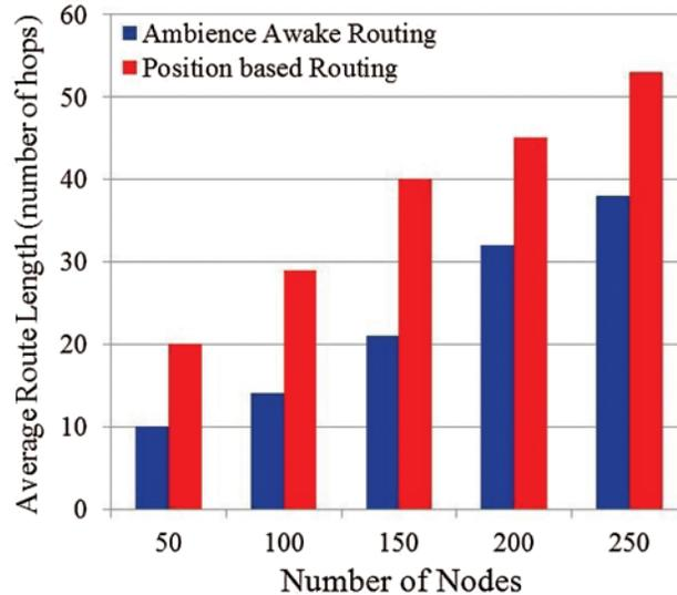
**Figure 5:** Average route length computation based on number of nodes
