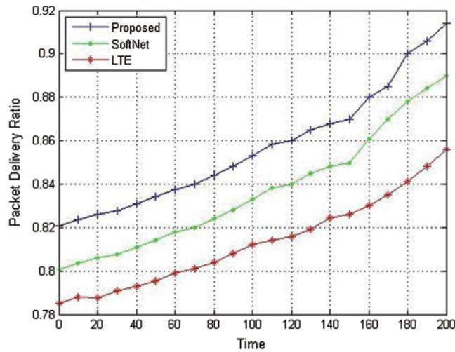
Figure 6: PDR variations with respect to simulation time
