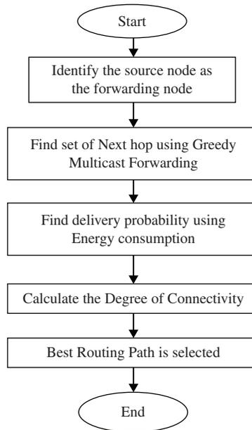
Figure 3: Flowchart for the routing process
