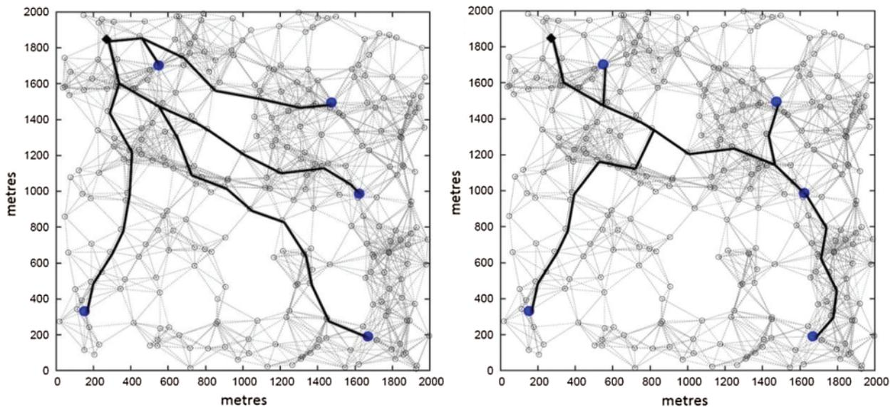
Figure 1: Packets split for forwarding ( $\lambda = 0$ ) and ( $\lambda = 1$ )
