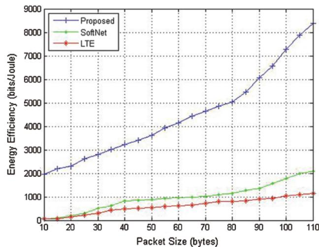
Figure 7: Energy efficiency for varying packet size (entities: 60)
