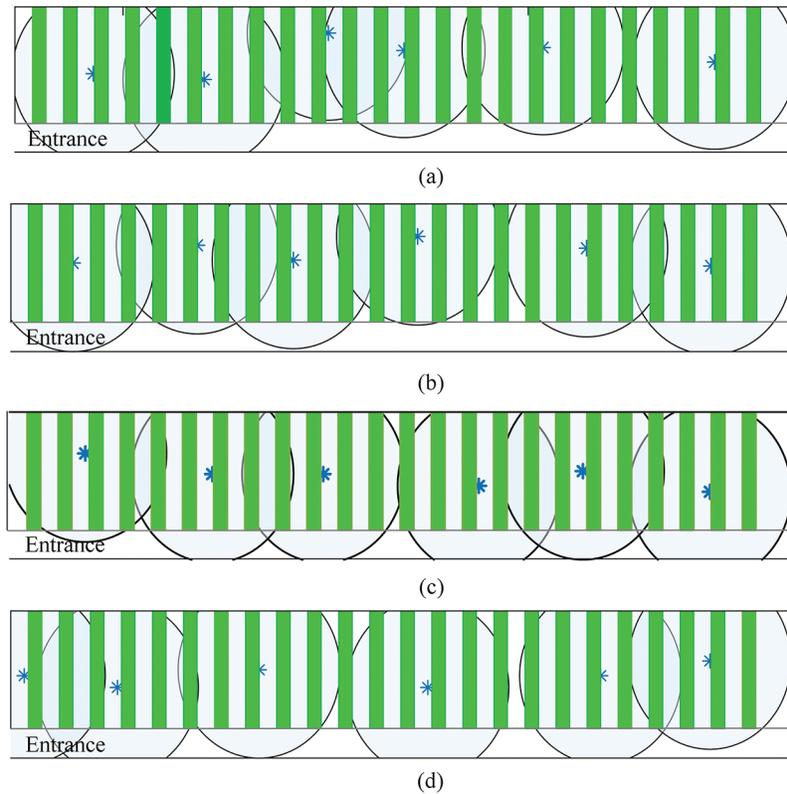
**Figure 10:** Network physical layout in the greenhouse at different sensor heights (a) Wireless network layout in greenhouse with antenna height of 0.5 m (b) Wireless network layout in greenhouse with antenna height of 1.0 m (c) Wireless network layout in greenhouse with antenna height of 1.5 m (d) Wireless network layout in greenhouse with antenna height of 2.0 m
