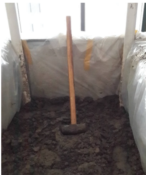
Figure 2: Filling earth material in the model tank
