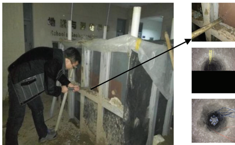
Figure 3: Implantation of the freezing tube and the inbuilt sensors
