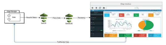
Figure 7: Illustration of data flow from edge manager to Vue.JS framework
