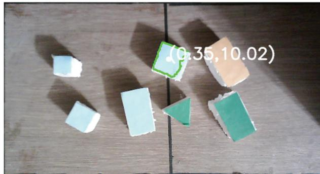
**Figure 15:** Sample output of size sorting where we are selecting for a large sized square object. Color has been set to blue and shape is set to square. So, selected object is a large blue square
