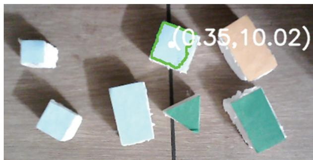
**Figure 14:** Sample output when color sorting is done and blue object is selected. Shape is set square and size is set to large, So, large blue square is targeted
