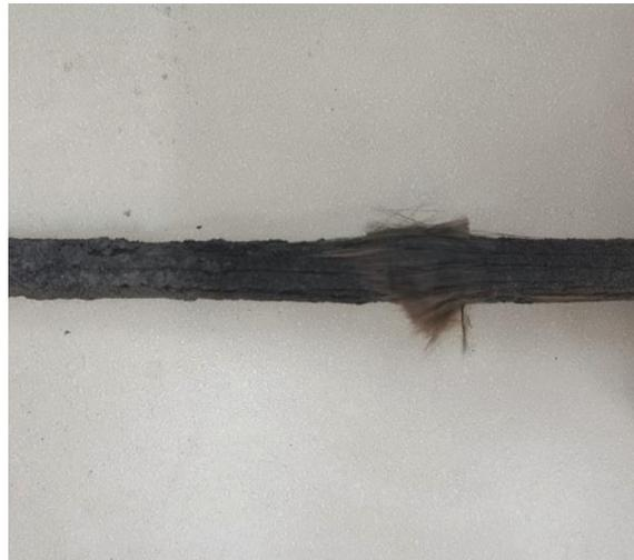
**Figure 8:** BFRP bar after 500°C
