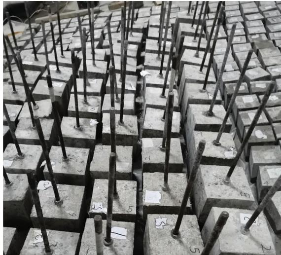
**Figure 2:** The specimens for pull-out tests in laboratory
