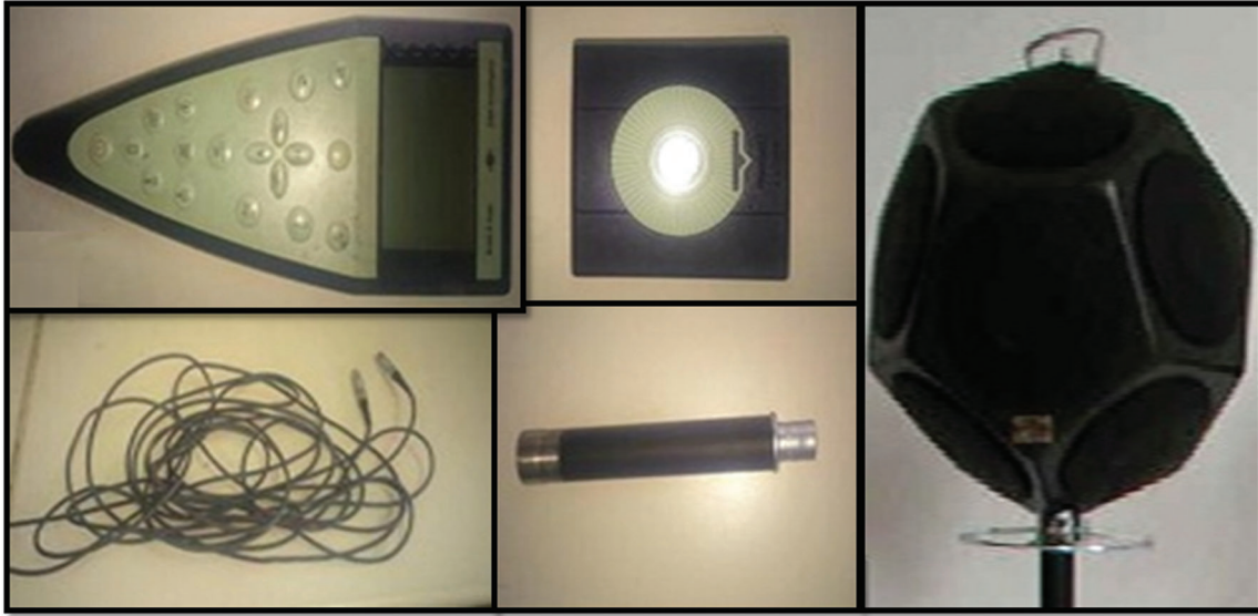
Figure 2: Sound level meter, sound level calibrator, microphone with preamplifier, cables and omni-power sound source
