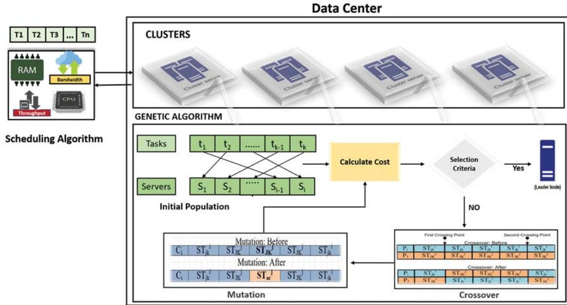
Figure 1: Proposed model of the genetic based leader election algorithm
