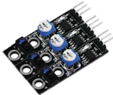
**Figure 5:** Tracking sensor
