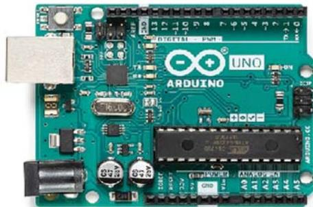
**Figure 4:** Arduino Uno based on the ATmega328P
