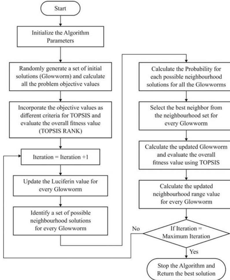
**Figure 2:** The flowchart of GSO algorithm
