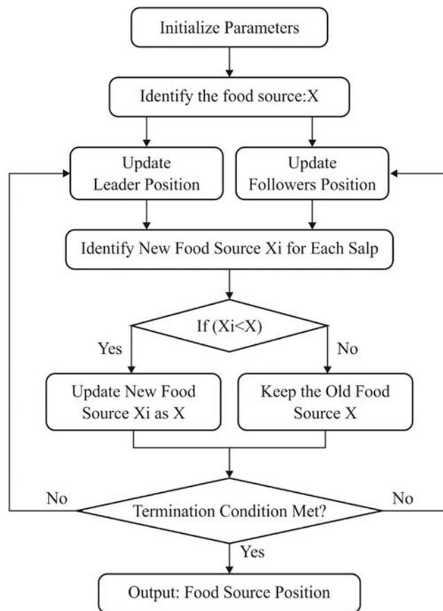
**Figure 3:** The flowchart of SSA model
