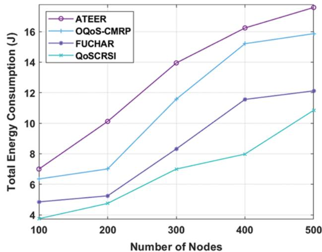
Figure 5: Results of QoS-CRSI model in terms of TEC
