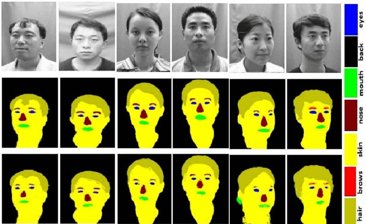
Figure 2: CAS-PEAL [29] images: row 1 has original images, row 2 the ground truth, and row 3 is segmented with the proposed segmentation framework
