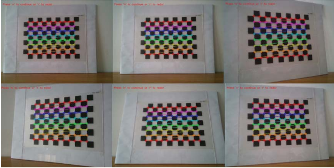
Figure 3: Corner detection diagram during camera calibration
