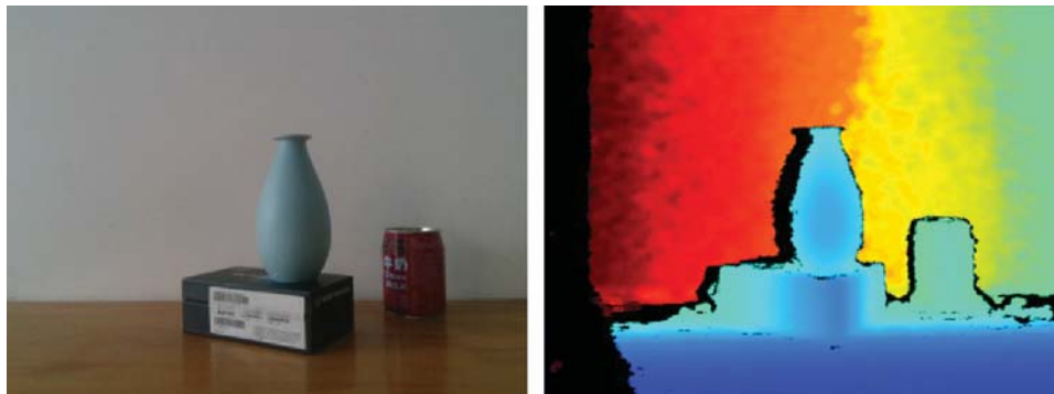
Figure 5: The aligned RGB map and depth map
