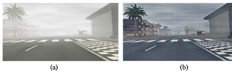
Figure 1: An illustrative example of an image defogging approach (a) the input fog image (b) the defog image
